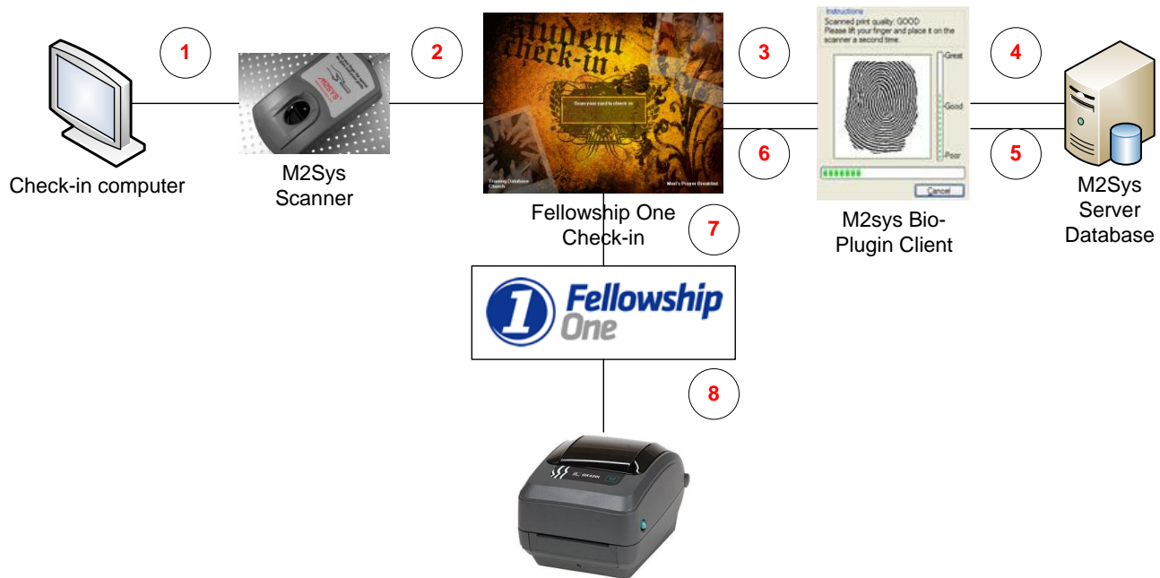
Figure 1- Fingerprint Scanning Process
