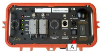
• **DO** check that you have a Red Tag Read LED (Lite Reader) Green Power, TX-A and TX-B Status Lights lit on the reader before starting your event. You should also have a Red/Orange Flashing LAN LED Light if you are plugged in to the Ethernet Port.
