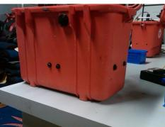
2. Remove the four Silver Phillips Screws from the four corners of the Control Panel.
