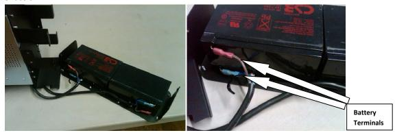
7. The batteries should lift out of the plate although they may be stuck slightly to the plate.
