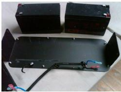
8. The replacement batteries can be acquired through Batteries Plus, Interstate Battery and online. The original part number varies based on the manufacturer but the Batteries Plus Part Number is; <a href="Werker#WKDC12-8NB">Werker#WKDC12-8NB</a>. This number can be crossed to other manufacturers through other dealers or websites. Below is a picture of an original CSB Battery and its' part number.
