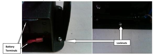
6. Remove the eight Silver Locknuts with a <u>7mm Wrench or Socket</u> and then gently lift up on the Silver Handles on the Control Panel and separate the Bottom Plate and batteries from the Chassis.
