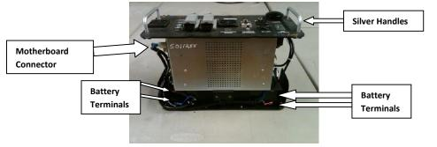
5. You will need to disconnect the two Red (Positive) and two Blue (Negative) Spade Connectors from the batteries before proceeding.
